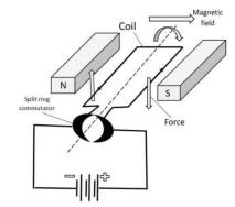
A DC motor requires DC electricity in order to function properly. The ball-bearing motor, which is still relatively new, & Michael Faraday's homopolar drive are two instances of pure DC designs. The two most prevalent forms of DC motors, brushed and brushless, convert the DC power they receive from an external or internal commutator to an alternating current (AC), making them not, strictly speaking, and DC machines.
